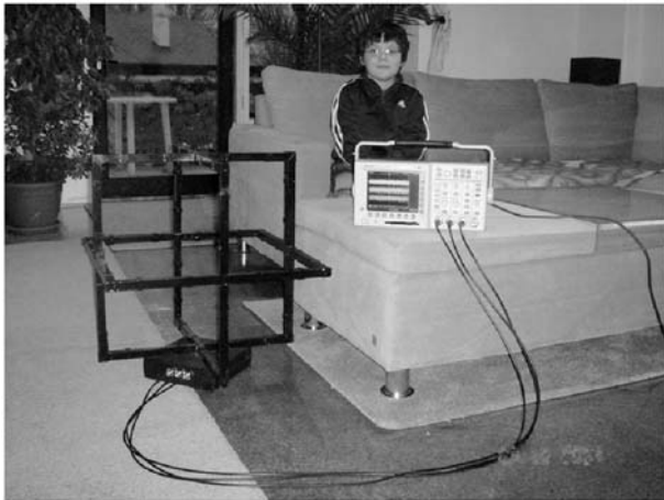
Fig. 1. The special-manufactured three orthogonal coils used for spot measurements, connected with oscilloscope by three shielded cables. Three coils have the dimensions 540 \times 600 \times 540 \text{ mm}^3 and the effective areas 15.3 \times 15.0 \times 14.7 \text{ m}^2 . Resistance is 10.6\text{--}11.0 \Omega and self-inductance 6.6\text{--}7.2 \text{ mH} in 120 \text{ Hz} . The relative error of an electric-parameter measurement is about 5%.
